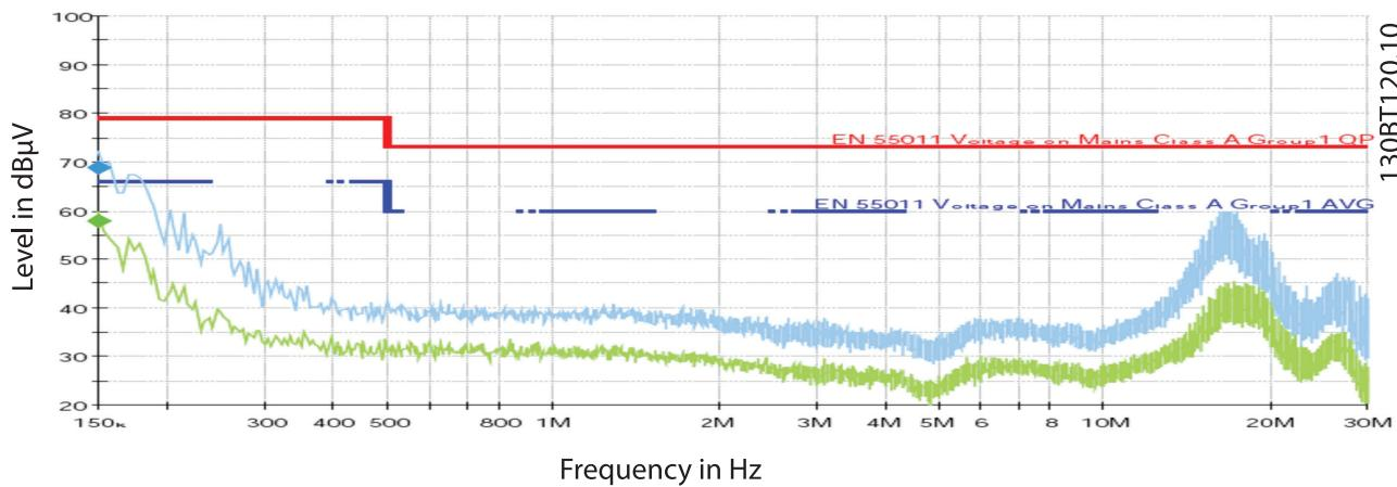
Illustration 3.8 Mains Line Conducted Noise, Sine-wave Filter
