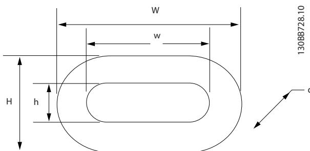
In normal operation the temperature is below 70°C. However, if the cores are saturated they can get hot, with temperatures above 70°C. Therefore it is important to use the correct number of cores to avoid saturation. Saturation can occur if the motor cable is too long, motor cables are paralleled or high capacitance motor cables, not suitable for frequency converter operation, are used. Always avoid motor cables with sector-shaped cores. Use only cables with round-shaped cores.
