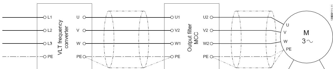
Illustration 5.3 Wiring Diagram
